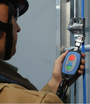
IBEX's patented continuous closed feedback loop employs a lightweight EasyClimb Controller. This simple wireless control connects the climber's body harness to the assist rope. The EasyClimb Controller transmits signals to the motor to maintain the desired level of assistance and to respond instantaneously to changes in climbing speed or direction. The field-tested controller's wireless signal seamlessly communicates climber behavior to adapt motor output for a consistent, reliable assist.
